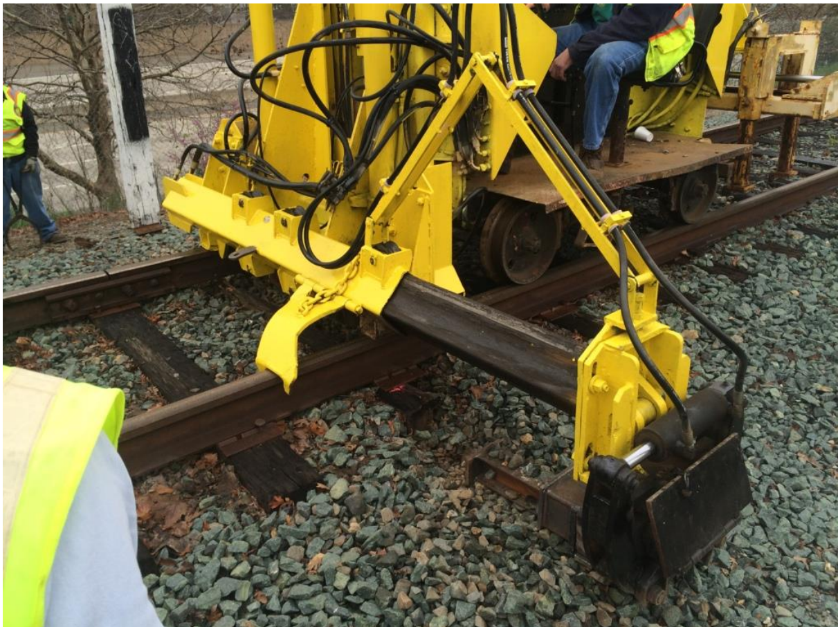
The custom-made ram attachment, designed by Alan and built by Cliff, is deployed on the 125 and works beyond expectations
